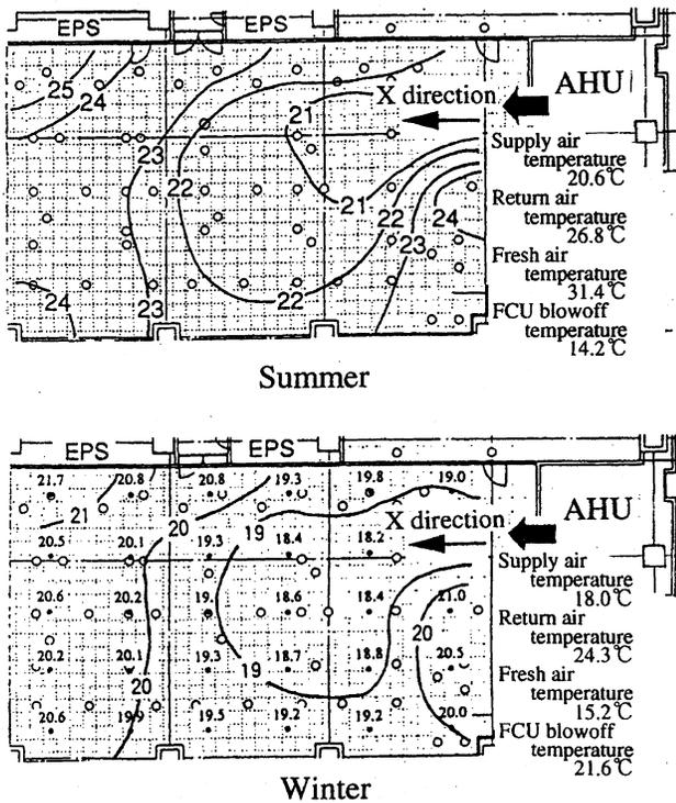
Figure 3 Air temperature distribution under the floor on a underfloor system floor.
