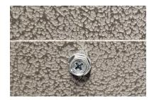
Use a Philips head or a 5/16-hex driver to unscrew the access door
