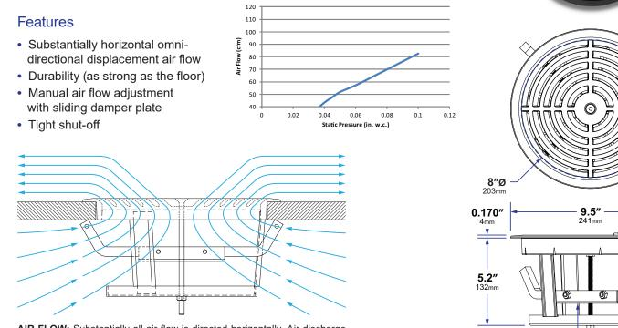
**AIR FLOW:** Substantially all air flow is directed horizontally. Air discharge pattern is designed so that velocity will decay below 40 fpm within a radius of 2' (0.6m) around the diffuser, delivering true displacement air distribution.
